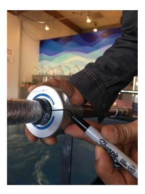
Screw in one side (do not tighten), measure to see 1 mm gap on the other side. If it is too wide of a gap, which means your Black pipe wrap tap is too thick. Remove some and cut and try again.
