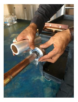
Apply Plastic Wrap around the Disc about 5 times
